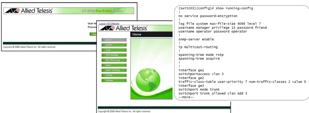
The image displays the web management interface of an Allied Telesis AT-9000 Eco-Switch Series switch. The interface includes a navigation menu with options like Home, System, Time, Port Settings, Port Mirroring, LACP, Static Trunking, VLANs, and Utilities. A terminal window on the right shows the output of the command `(switch3)(config)# show running-config`, displaying the current configuration of the switch, including system settings, user accounts, and interface configurations.
